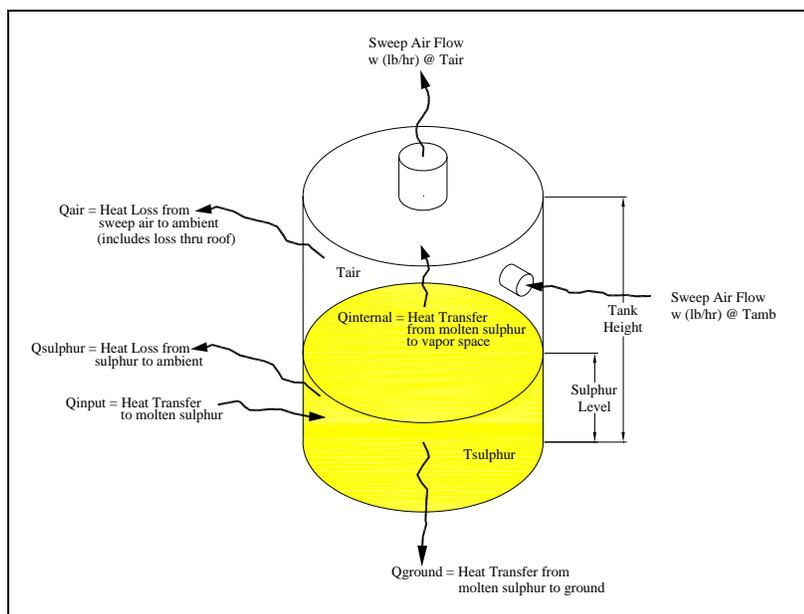
Figure 2 – Thermal Maintenance Model
