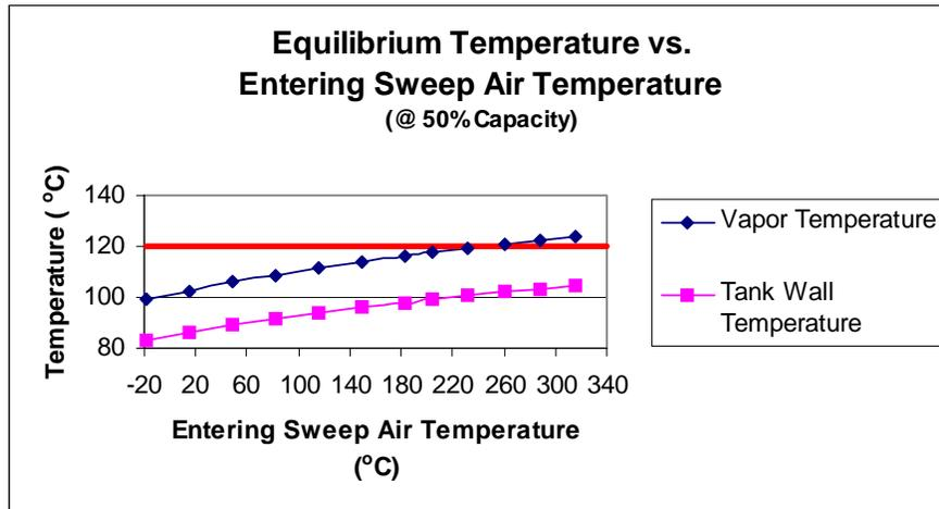
Graph 2 – Internal Vapor Temperature & Tank Wall Temperature vs. Entering Sweep Air Temperature
