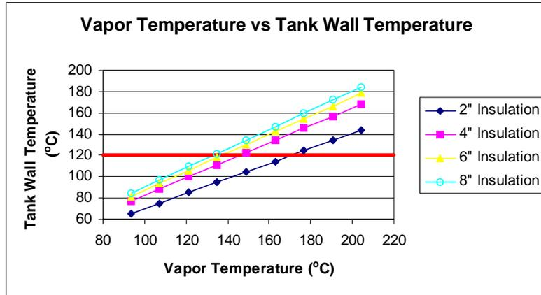
Graph 1 – Internal Vapor Temperature vs. Tank Wall Temperature
