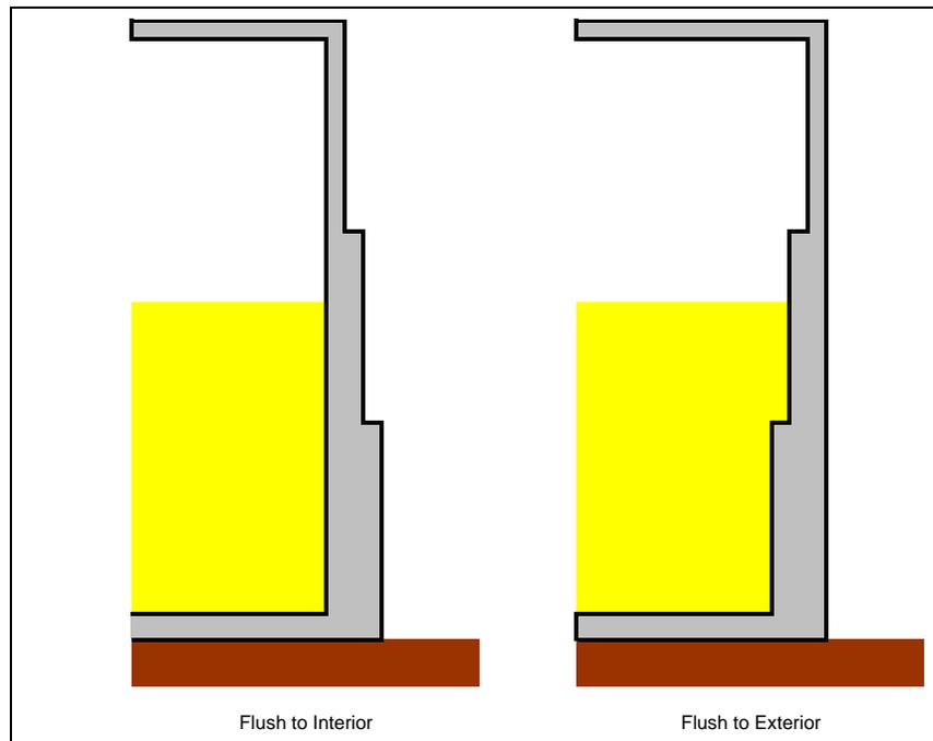
Figure 10 – Methods of Tank Side Wall Construction
