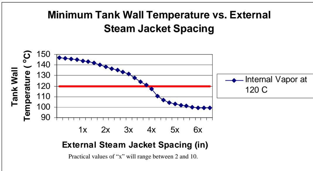
Graph 3 – Minimum Tank Wall Temperature vs. External Steam Jacket Spacing
