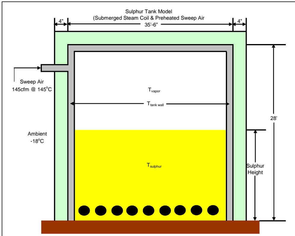
Figure 4 – Scenario 2, Sulphur Tank with Steam Coil Heating and Sweep Air @ 145°C
