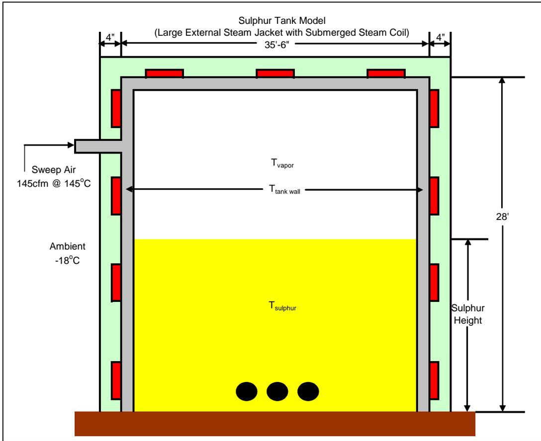
Figure 7 – Scenario 3, Sulphur Tank with Steam Coil Heating with Large External Steam Jackets and Sweep Air @ 145°C
