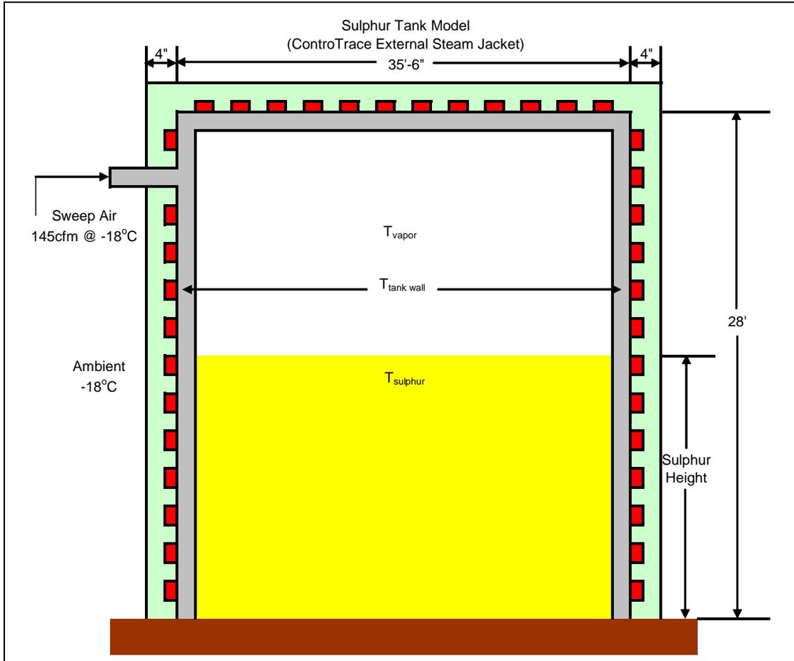
Figure 9 – Scenario 4, Sulphur Tank with ControTrace External Steam Jackets and Sweep Air @ -18°C
