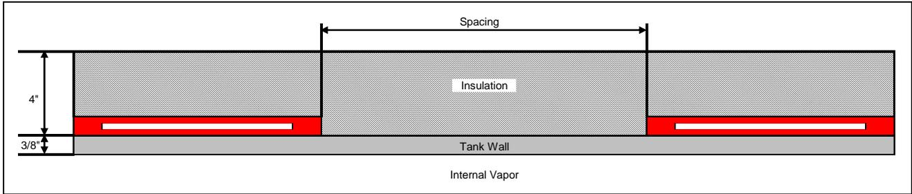
Figure 5 – Cross Section View of Tank with External Steam Jacket.
