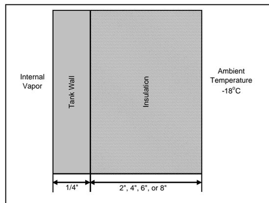
Figure 1 – Cross Section View of Storage Tank in Vapor Space
