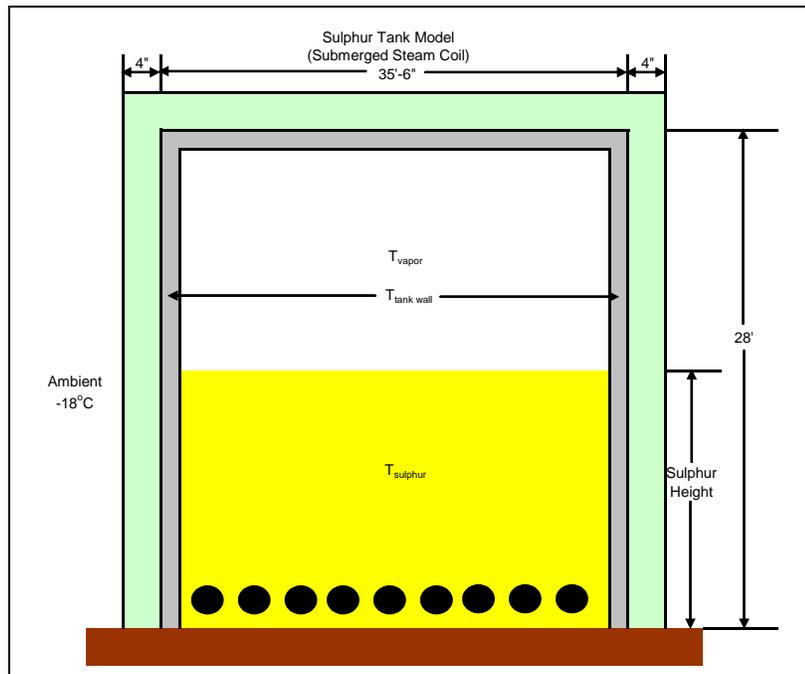
Figure 3 – Scenario 1, Sulphur Tank with submerged steam coil
