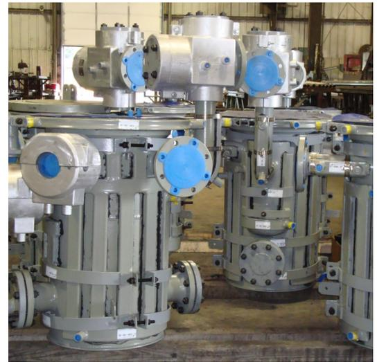
*Jean Gaulin Refinery's S<sub>x</sub>Seal™ 2000 sulfur sealing devices, shown in production at CSI*
